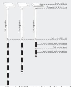
Figure 3 Example of PYCNO sensor probe length which allows soil moisture and temperatures and different depths (PYCNO, 2020)
