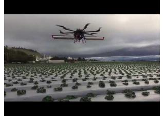
Figure 8 Parabug drone releasing beneficial insects for biocontrol over a range of crops. Click image for video. (Parabug, 2018)
