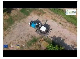
Figure 7 Rovitis 4.0, an autonomous vineyard sprayer. Click image for video. (Pantano, 2019)
