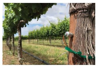
Figure 4 FloraPulse installed on a grapevine trunk, showing the sensor casing and wires (Picture by Michael Santiago in Growing Produce, 2019)
