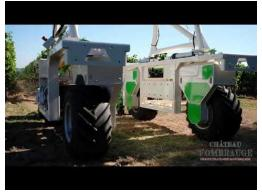
Figure 6 TED, an autonomous vineyard weeder. Click image for video (Naïo Technologies, 2018).
