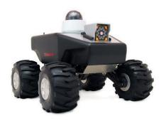
Figure 5 VINBOT, an autonomous yield estimation and NDVI mapping vineyard robot (VINBOT,2020)
