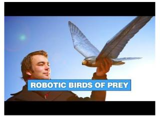
Figure 9 Robird bird scaring drone, designed to mimic the flight and size of a peregrine falcon. Click image for video. (Oddity Mall, 2017)
