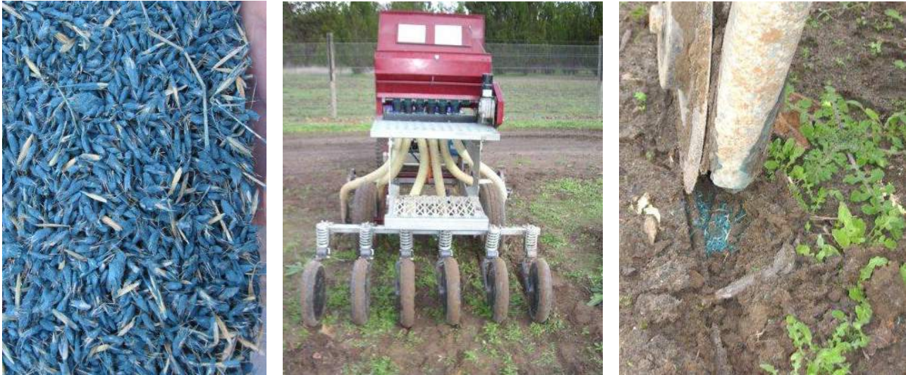
Figure 19. Pelletised wallaby grass ready for seeding (left), rear view of the seed drill. The rear wheels ensure the seed is firmly bedded into the soil (middle), and wallaby grasses planted to a depth of 0.5 to 1 cm (right).
